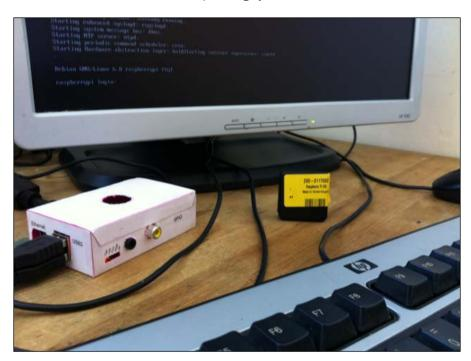
The preceding image shows a Raspberry Pi in the Punnet with monitor, keyboard, and mouse.
