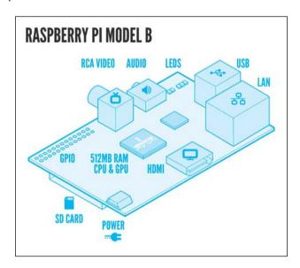
The preceding image is a schematic diagram of the Raspberry Pi from Raspberry Pi Foundation (http://www.raspberrypi.org).
