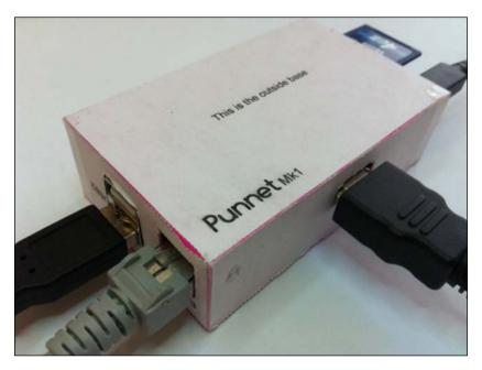
The preceding image shows the Punnet in use. A printed Punnet was glued to pink card stock before folding. The card stock added strength and stability to the case.
