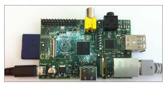
The preceding image shows a Raspberry Pi with an SD card, a network, and power cables.
